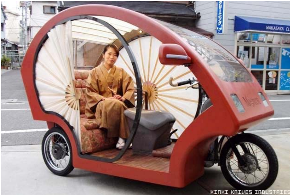
The "Meguru" is a three-wheeled, three-seat compact vehicle whose single lithium-ion battery allows for a maximum speed and range of 40 kilometers (25 miles) per hour, although the number of batteries could be increased for a longer ride.
